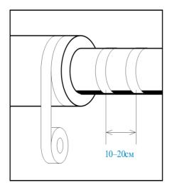
After the IQ PIPE cable has been attached to the metal or plastic pipe, so that every part of the cable system is in contact with the pipe, cover it with fiberglass, preformed foam or other inflammable insulation of ½" thickness.
